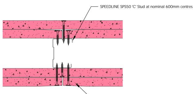
2 layers of 15mm British Gypsum Gyproc FireLine fixed with SPEEDLINE Drywall Screws at 300mm centres (200mm centres at external angles). Ref to table for fixing length.
